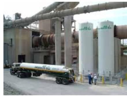
and thereby raises the level of possible alternative fuel substitution. The resulting improved kiln control and stability with oxygen enable operators to maintain feed rates and burn more consistently than with air alone.
